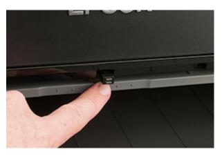
To activate the single sheet path, push on the gray bar above the paper output tray. This will cause the tray to lower and extend. Follow the printer's on-screen instructions to load your media.
