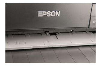
**WARNING** - The front feed in fine art mode is a bit unpredictable. The internet is peppered with reports of misfeeds and problems getting it to work. The root cause is a plastic lip near the back of the feed path as the paper curves up and out through the back door. Heavier, stiffer paper crashes into the lip instead of going over. Chaos ensues.
